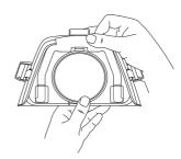
4. Refit the O-ring in the channel of the tub plate.
